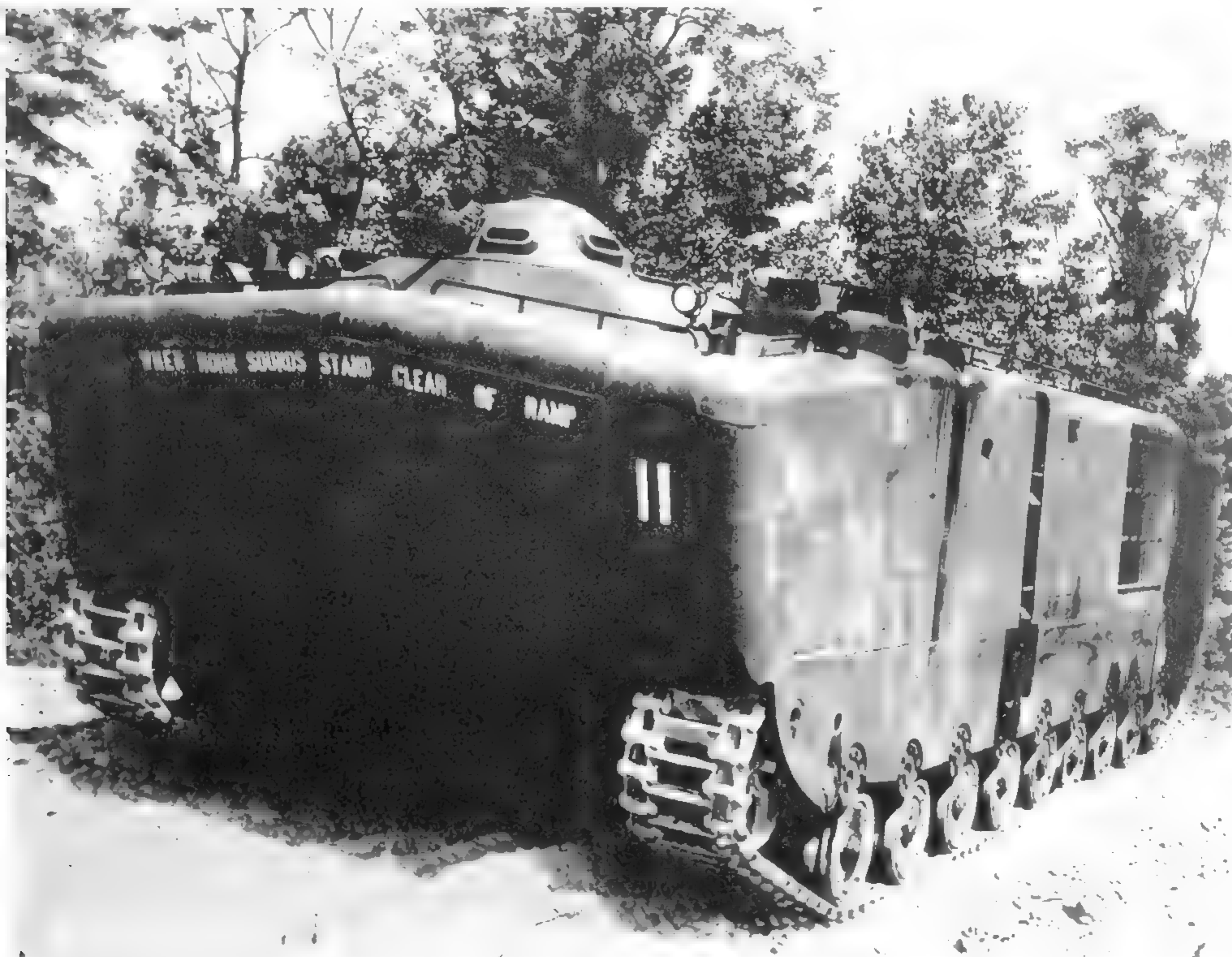
This LVTP5 has been equipped with the .30-caliber machine gun turret on the top. Among the improvements of the LVTP5 was its totally enclosed cargo and personnel compartment. (Photo courtesy of the Patton Museum)
